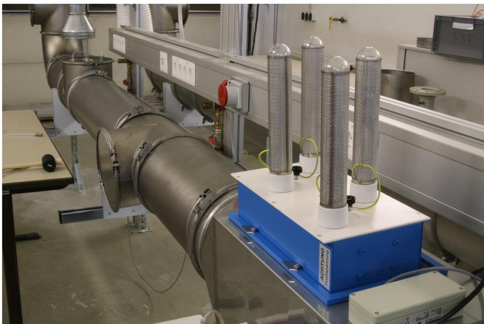
Figure 1: ionair ionization module.
