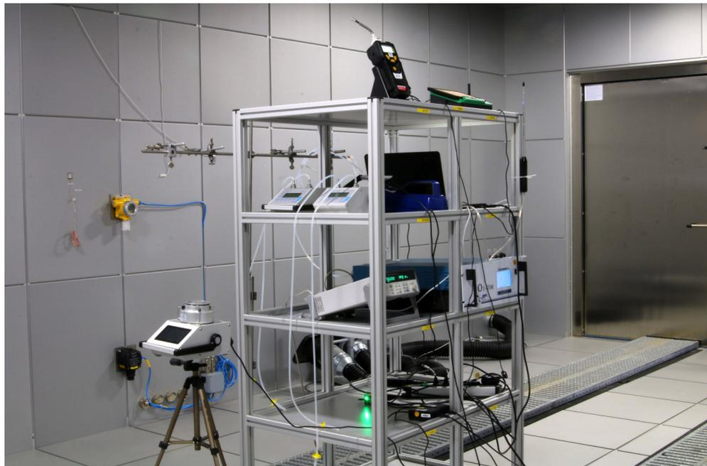
Figure 3: Setup of the sensor technology and air sampler in the IATC room.
